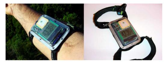
Prototype of fully waterproof case for GT31/GT32. The case has wide angle of view and 2 straps. When you use Speed Genie there is no need to push any buttons when you measure your average speeds. Turning on/off and basic manual operation is done using a magnet. Charging and access to SD card requires disassembling the case using a screwdriver.
